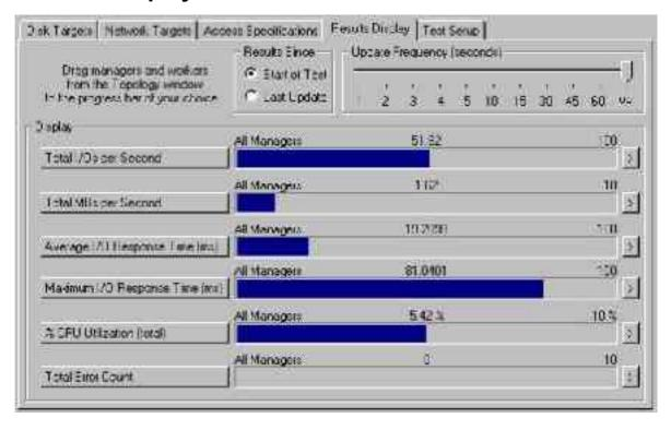
The Results Display tab displays performance statistics while a test is running. You can change the settings of all controls in the Results Display tab while the test is running. Any changes you make take effect immediately.
