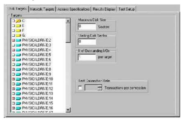
The Disk Targets tab lets you see and control the disks used by the disk worker(s) currently selected in the <u>Topology</u> panel.
