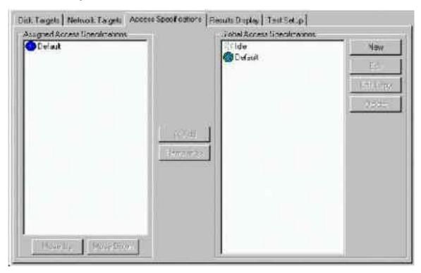
The Access Specifications tab lets you control the type of I/O each worker performs to its selected target(s). Each named access specification controls:
