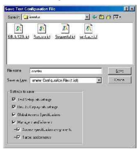
Pressing the Save Test Configuration File toolbar button brings up the Save Test Configuration File dialog. You may choose which settings to include in the saved file. For further details, see the <u>Save Test Configuration File – Reference</u> section.
