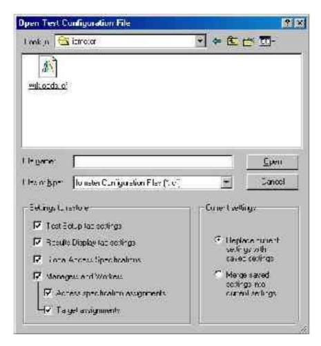
Pressing the Open Test Configuration File toolbar button brings up the Open Test Configuration File dialog. In addition to the following, also see the <u>Iometer Configuration File (.icf)</u> section for further information.
