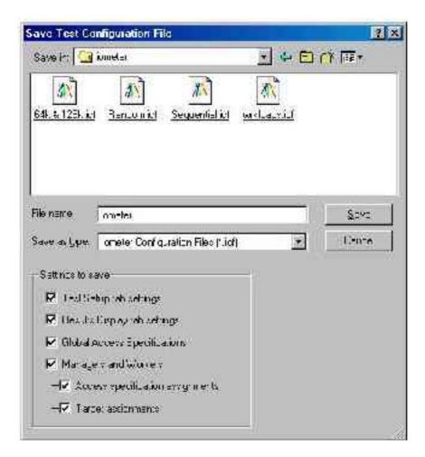
Pressing the Save Test Configuration File toolbar button brings up the Save Test Configuration File dialog.
